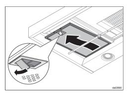
Open the grease filter lock, lower the grease filter slightly, unhook it at the back, and take it out.
